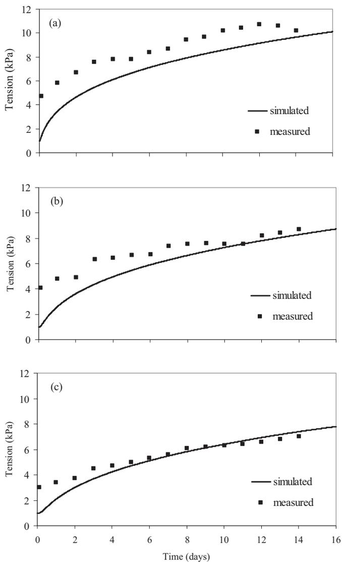
**Fig. 4.** The change in tension post saturation after the lucerne crop was removed at a) 300 mm b) 600 mm and c) 900 mm depths. The solid lines show the simulations from Hydrus-1D.
