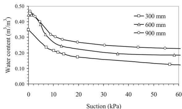
Fig. 1. The draining water release characteristic at 300, 600 and 900 mm depths.
