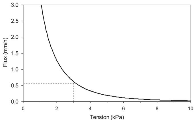
**Fig. 5.** The flux rate as a function of soil tension at 600 mm depth from the Hydrus simulation of a draining profile. The dotted line represents the sensitivity limit of the WFD.
