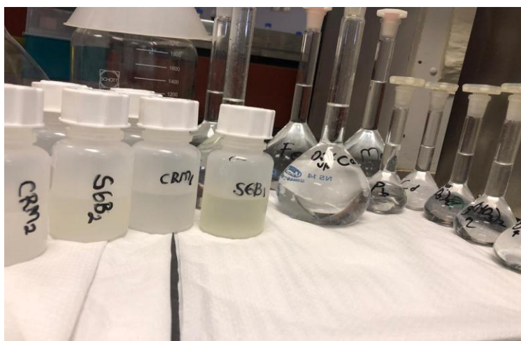
Figure No. 2: Samples of microwave digestion (analytes in plastic bottles) and prepared working standards
