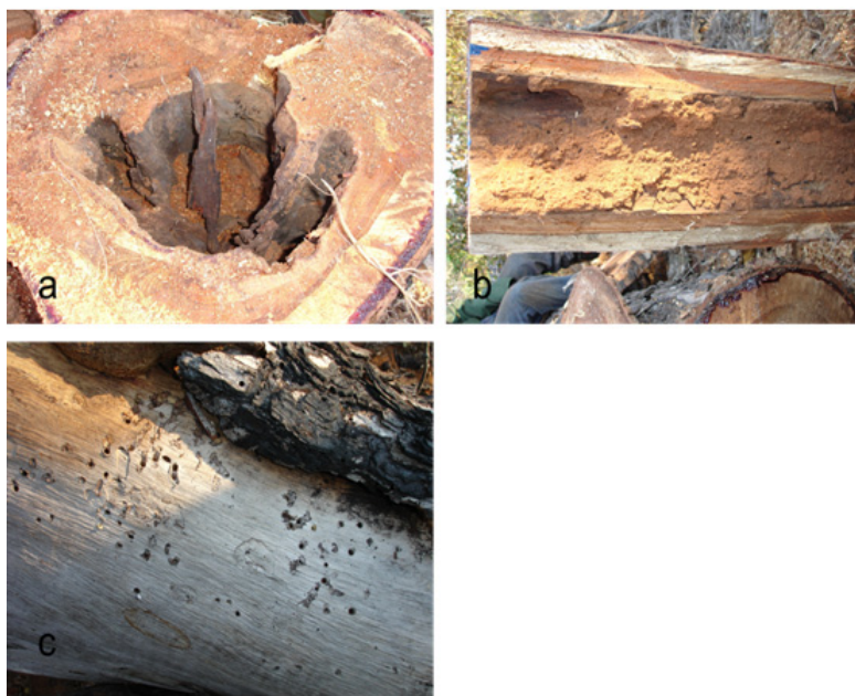
Figure 1. Damage by termites (a and b) through tunnelling and Cerambycidae (c) tunneling in the sapwood
