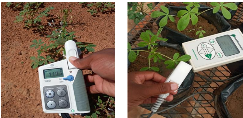
Figure 3.1: Measurements of chlorophyll content (left) and stomatal conductance (right) on leaves of Cleome gynandra L.
